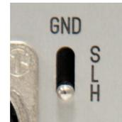
Lower position: (H)ard-ground: The ground pin is conductively connected to the ground center of the internal circuit.
