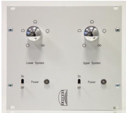
The power supply is built as a module to fit into any 19 inch studio rack next to pre-amps and effects or to be used as a stand alone device. It contains two separated supplies for each microphone. Thereby the VM1S can be used as a single microphone and in stereo mode the highest possible crosstalk rejection is achieved.
